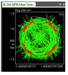
Figure 1. QPSK signal with emulated phase noise
