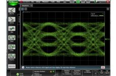
Figure 2. PAM-4 signal at 56 GBaud
