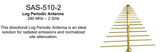
Frequency Range: 290 MHz - 2000 MHz Antenna Factor: 14 - 32 dB/m Gain: 6.5 dBi Maximum Continuous Power: 1000 Watts Maximum Radiated Field: 200 V/m Pattern Type: directional 3dB Beamwidth (E-Field): 45° 3dB Beamwidth (H-Field): 100° Impedance: 50  $\Omega$ VSWR: 1.45:1 typ. (2.2:1 max) Connector: N-Type, Female Mounting Base: 1/4 x 20 Thread, Female
