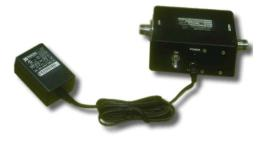
Frequency Range: 20 MHz – 7 GHz Gain (typical): 30 dB Gain (minimum): 24 dB Flatness: +/- 5.0 dB Noise Figure: 5.0 dB Maximum Input Power -10 dBm Input VSWR (typical): Less than 2.2:1 Output VSWR (typical): Less than 1.8:1 Connector: N-Type, female
