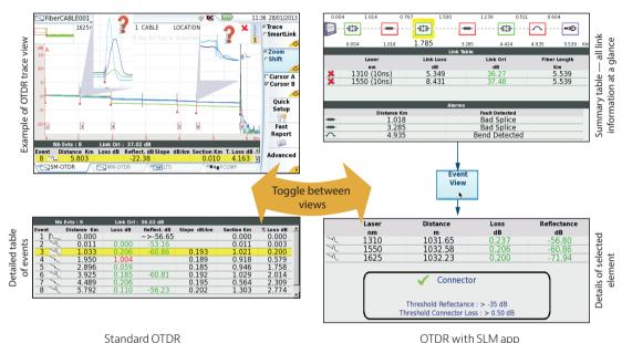
SLM analyzes and identifies events of any OTDR trace, new or old. It represents them as simple icons with immediate pass/fail information based on user-defined or IEC/TIA standards thresholds. It explicitly names the type of optical element such as a splice or connector.
